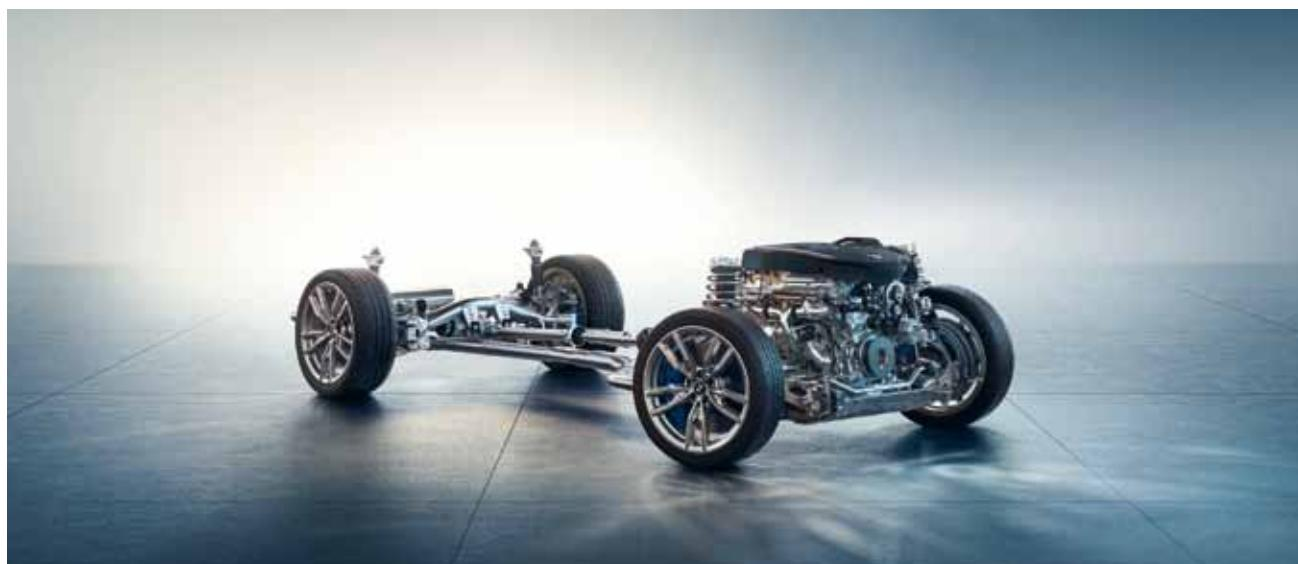
M Sport suspension<sup>1</sup> – which includes a suspension which is lowered by 10 millimetres – is characterised by more athletic suspension settings with tighter damper settings. It also features a moderately higher spring constant and harder stabilisers. Combined together, they result in an even more direct suspension design, which enables a distinctly sporty driving style.
