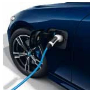
With the standard charging cable (mode 2) for domestic socket outlets, you can conveniently charge your BMW's high-voltage battery at domestic sockets.
