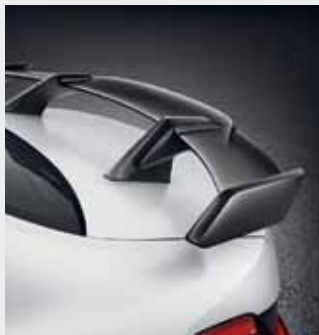
o The M Performance rear spoiler with aerodynamic cut-out is made from 100 percent high-quality carbon fibre and creates a distinctive motorsport look at the rear of the vehicle.
