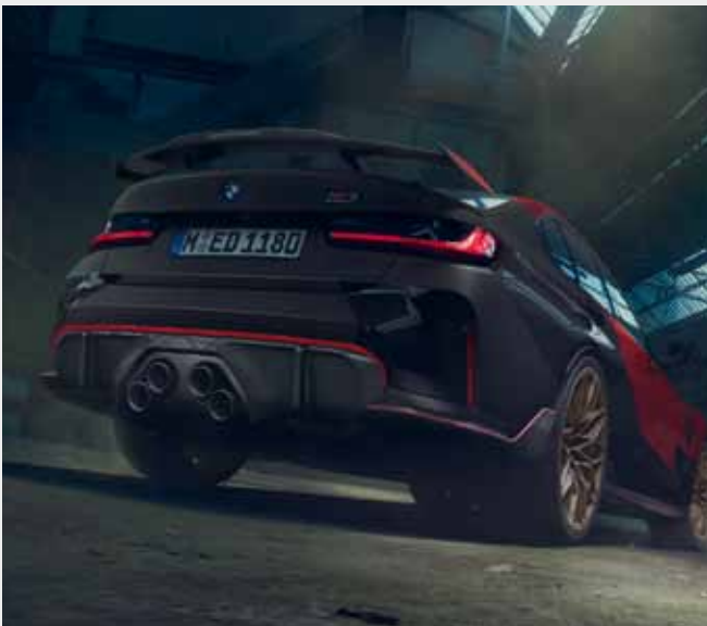
o The M Performance rear spoiler with aerodynamic cut-out is made from 100 percent high-quality carbon fibre and creates a distinctive motorsport look at the rear of the vehicle.
