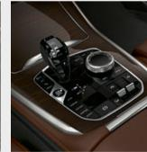
■ The 8-speed Steptronic Sport transmission offers incredibly sporty gear changes, both automatically and manually via the gearshift paddles or selector lever.
