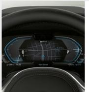
The plug-in hybrid-specific instrument cluster provides information on, among other things, the status of the vehicle's electric readiness, the charge level of the battery and average electrical consumption.
