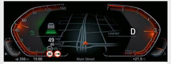
☐ The automatic Speed Limit Assist\* adapts the Active Cruise Control dynamically to upcoming speed limits. These are determined along the probable route by the navigation system and checked by the camera. The information provided is continuously updated by the entire fleet.
