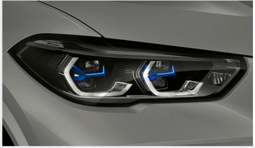
☐ In laser high-beam mode, BMW Laserlight in a unique X design illuminates a range of up to 500 m, nearly twice as far as that of conventional headlights. Better visibility in the dark significantly increases safety. The blue X signature and the "BMW Laser" lettering underline the vehicle's technological standards.
