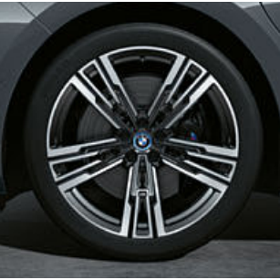
21" M light alloy wheels Star-spoke style 908 M Bicolour Jet Black with mixed tyres, gloss-lathed, wheel size front 9J x 21 with 255/40 R21 tyres, wheel size rear 10.5J x 21 with 285/35 R21 tyres.
