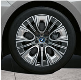
20" aerodynamic wheels 906 Bicolour Dark Grey 3D buffed with mixed tyres, gloss-lathed, wheel size front 9J x 20 with 255/45 R20 tyres, wheel size rear 10.5J x 20 with 285/40 R20 tyres. 1
