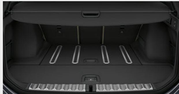
□ In addition to the electric remote backrest unlocking, the luggage compartment package also includes practical slide and anti-slip rails, depending on the engine version, for easy loading into the luggage compartment or for securing heavy items of luggage during the journey.
