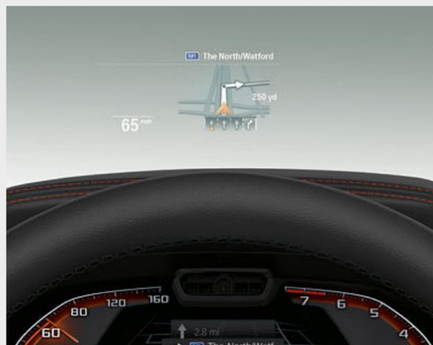
□ The large full-colour BMW Head-Up Display<sup>1</sup>\* projects information relevant to the journey directly into your field of vision, thereby allowing you to fully concentrate on driving. Information such as the current speed, navigation directions, Speed Limit Info including no-overtaking indicator, along with telephone and entertainment lists are displayed, depending on the equipment.
