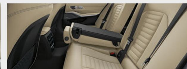
■ The Through-loading system includes rear seat backrests that can be divided in a 40:20:40 ratio for the greatest possible flexibility. For example, two passengers can be seated comfortably in the rear, while long objects such as ski and snowboard bags can be transported at the same time. The two cupholders in the centre armrest are very practical.
