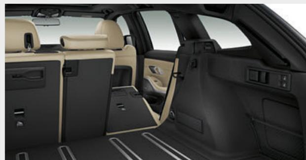
□ The storage compartment package includes a fold-down compartment on the driver's side of the instrument panel, nets on the back of the front-seat backrests, as well as two USB ports with charging function in the rear centre console. There is also a storage net on the left and right side for smaller items and a multipurpose hook in the luggage compartment.
