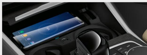
□ Telephony with wireless charging<sup>2</sup> incorporates a wireless charging dock and a second microphone for a better hands-free voice quality for you and your front passenger. A roof aerial connection improves mobile reception. Two mobile telephones and an audio player can be connected simultaneously via Bluetooth. Also included is the technical capacity for a WiFi hotspot<sup>3</sup>.
