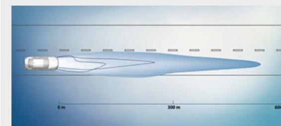
□ The Adaptive **BMW Laserlight** extends the maximum illumination range in high-beam mode to up to 530m.
