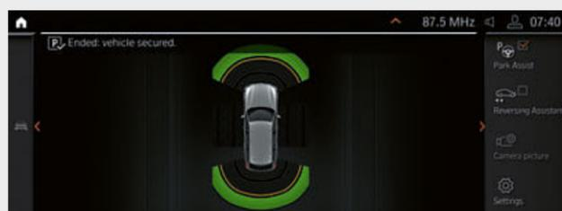
□ Parking Assistant Plus\* makes parking and manoeuvring the vehicle easier. It features among others the Surround View system including Top View, Panorama View, Remote View 3D, as well as a lateral parking aid, the emergency braking function Active Park Distance Control, Parking Assistant with linear guidance and Reversing Assistant.
