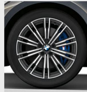
■ 18" M light alloy wheels Double-spoke style 790 M Bicolour Orbit Grey with mixed tyres, burnished, front 7.5J x 18 with 225/45 R18 tyres, rear 8.5J x 18 with 255/40 R18 tyres.
