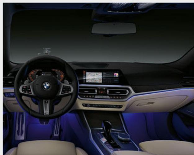
□ Ambient light, including Ambient contour lighting in the front and rear doors, creates a relaxed, cosy lighting atmosphere in the interior. The six dimmable lighting designs also include a dynamic function in four applications. The Welcome Light Carpet illuminates the area in front of the vehicle doors when entering and exiting.
