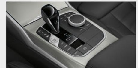
■ In eDrive drive, the drive modes HYBRID, ELECTRIC, and BATTERY CONTROL can be selected using specific control buttons.
