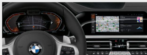
The BMW Live Cockpit Professional\* with navigation function<sup>5</sup> includes two high-quality displays consisting of a high-resolution 10.25" Control Display that can be operated by touch and a fully digital 12.3" instrument display. The BMW Operating System 7 can also be operated via the iDrive Touch Controller.
