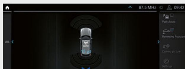
□ The Reversing Assistant\* stores the last 50m of the driven path in forward travel up to a speed of 35km/h, so that it can be retracted if required.
