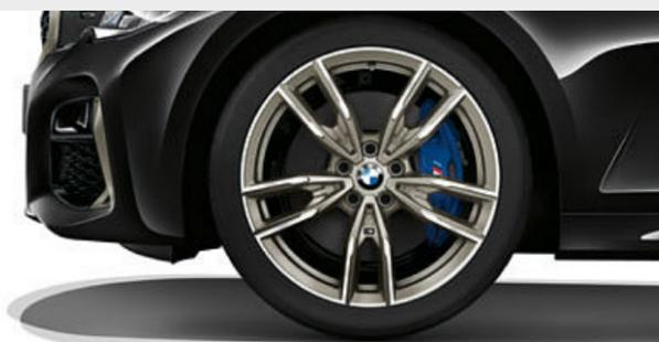
□ 19" M light alloy wheels Double-spoke style 792 M Bicolour Cerium Grey with mixed tyres and runflat tyres<sup>2</sup>\*, burnished, front 8J x 19 with 225/40 R19 tyres, rear 8.5J x 19 with 255/35 R19 tyres.
