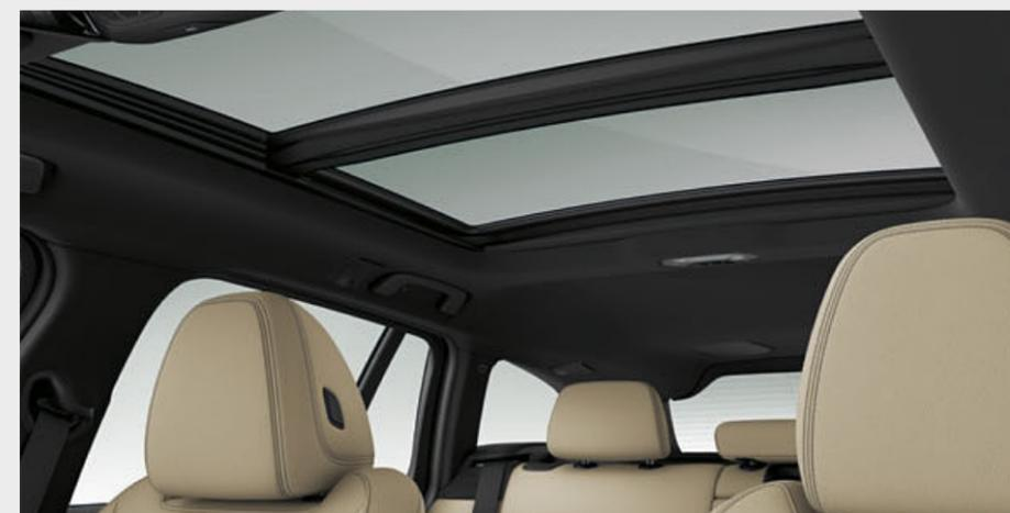
□ When open, the Panorama glass roof provides a great deal of fresh air. Closed, it creates a bright, light-flooded atmosphere in the interior. It opens and closes completely automatically at the push of a button or with the vehicle key, and is equipped with slide and lift functions, electric roller sunblind and wind deflector.
